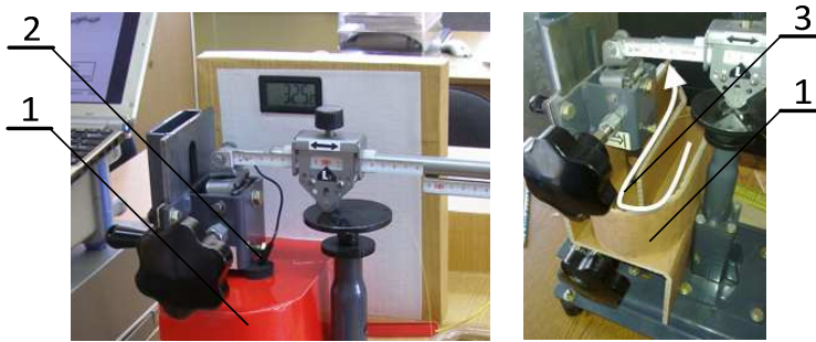
Fig. 2. Thermal chamber providing strain measurement in various temperature conditions: 1 - chamber enclosure, 2 - thermometer probe, 3 - flow direction of input air, with a regulated temperature.
